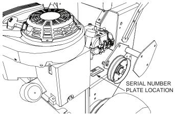
Figure 1-1. Mower Serial Number Plate Location
